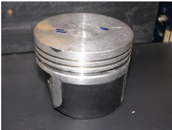
Fig. 2. View of the piston with an applied layer of nanotubes prior to engine test.
