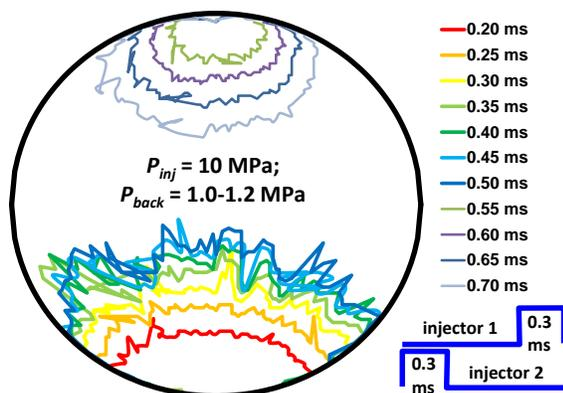
**Figure 14.** Fuel spray atomization in the RCM during a sequential fuel injection by two injectors.
