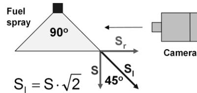
**Figure 3.** A method of determining linear and radial fuel spray penetration.
