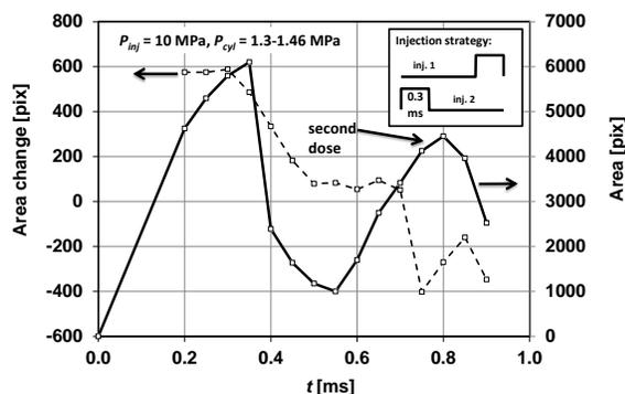
**Figure 15.** Change of fuel spray area during two part injection in Rapid Compression Machine.
