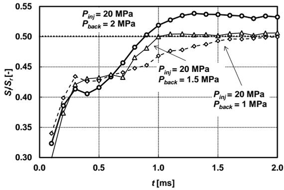
**Figure 5.** Linear and radial fuel spray penetration for one fuel injection (variation of back pressure);  $t_{inj} = 0.6$  ms.
