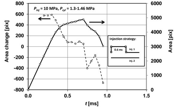
Figure 12. The change of area of fuel stream during single dose injection in Rapid Compression Machine.
