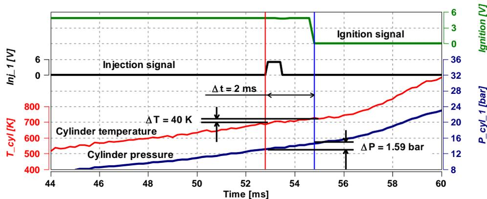
**Figure 10.** Pressure and temperature change during one-piece injection to RCM.
