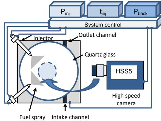
**Figure 1.** The Constant Volume Chamber with optical system for measuring fuel atomization.
