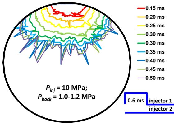
Figure 11. Fuel spray atomization in the RCM during a one fuel dose injection.
