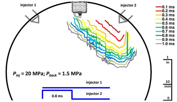
**Figure 6.** Fuel atomization sequence of a single fuel dose in the constant volume chamber (colors denote subsequent fuel spray penetrations (determined via DaVis)).
