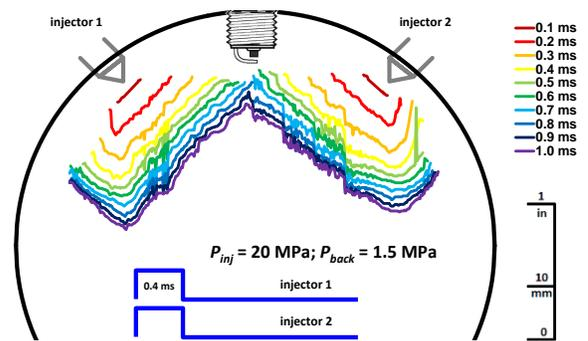
**Figure 8.** Fuel spray atomization in the constant volume chamber during a simultaneous injection of fuel via two injectors.
