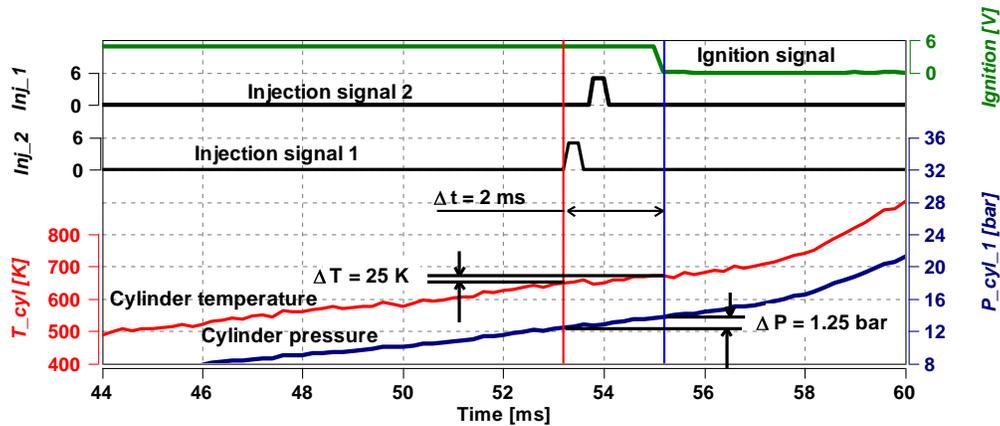
Figure 13. Pressure and temperature change during two-piece injection to Rapid Compression Machine.
