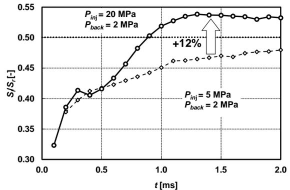
**Figure 4.** Linear and radial fuel spray penetration for one fuel injection (variation of fuel pressure);  $t_{inj} = 0.6$  ms.
