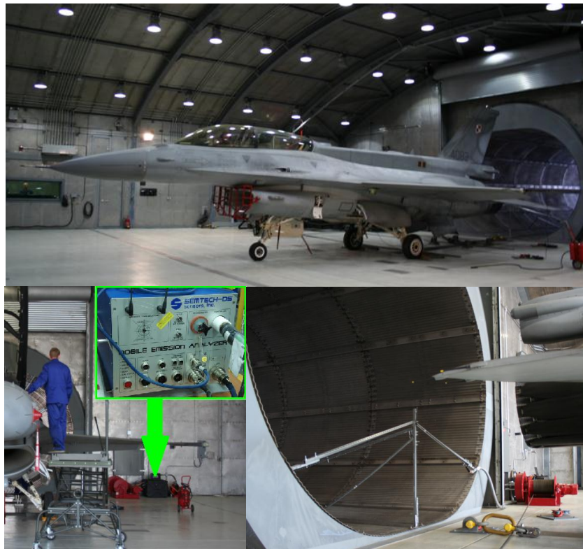
Figure 4: Location of the measuring probe and the analyzer.
