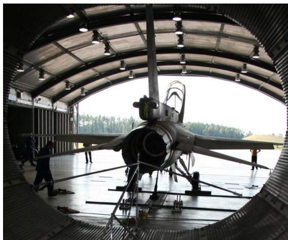
Figure 8: Location of the measurement probe in the axis of the exhaust gas flow leaving the engine
