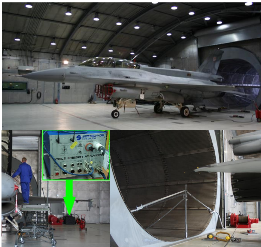
Fig. 3. Location of the measuring probe and the analyzer.
