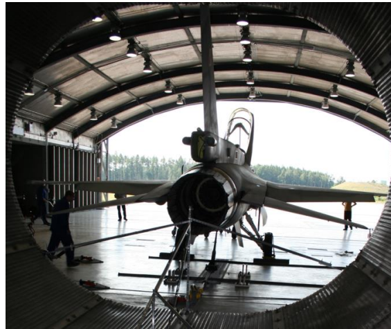
Fig. 8. Location of the measurement probe in the axis of the exhaust gas flow leaving the engine.
