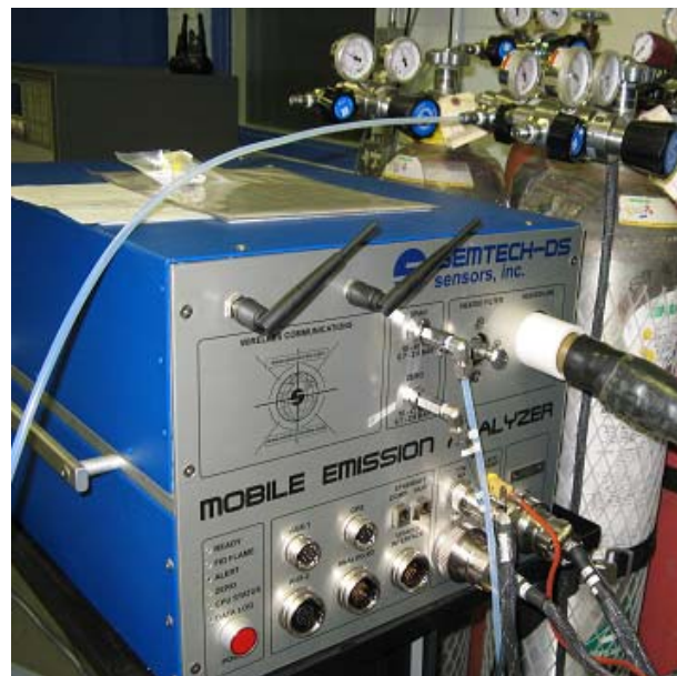
Fig. 4. View of the exhaust emission analyzer.
