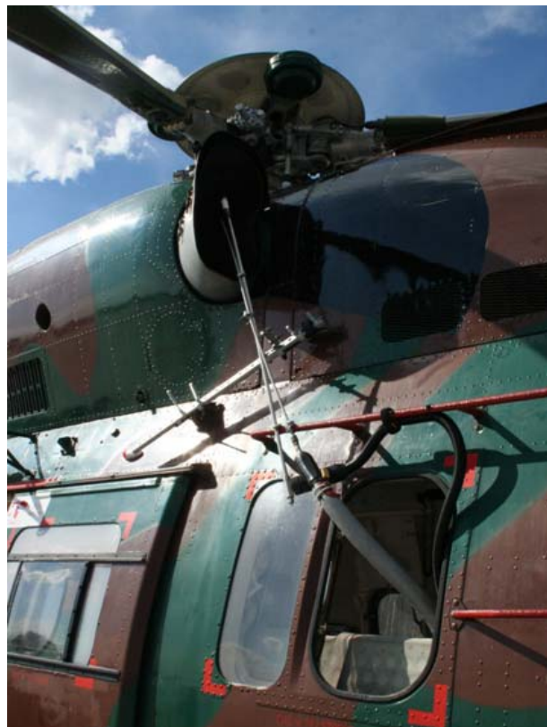
Fig. 3. Placement of the exhaust gases probe.
