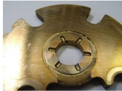
Fig. 3. View of scraped surface of bearing
