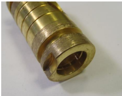
Fig. 9. View of faded bearing (dry friction)
