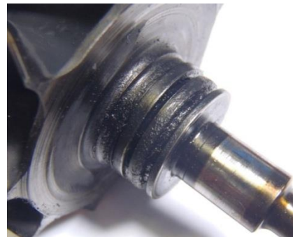
Fig. 5. View of rotor's shaft with ring seals becoming stuck in their grooves
