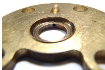
Fig. 11. View of bearing with hot tracks
