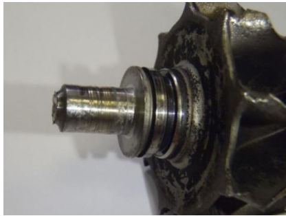
Fig. 2. View of broken rotor's shaft necks with deep scrapes
