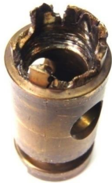
Fig. 7. View of damaged bearing
