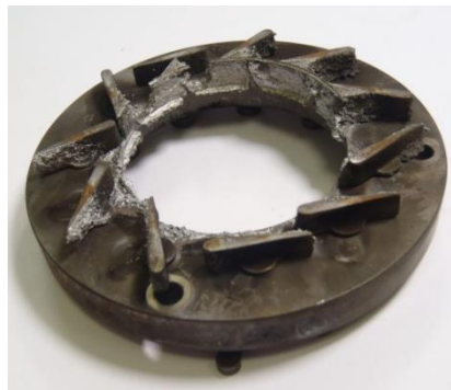
Fig. 12. View of exhaust steering wheel with contaminations on surface
