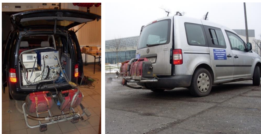
Figure 2: Vehicle with installed apparatus for measuring emission of exhaust gases in real traffic conditions.
