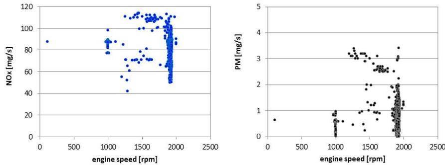
Figure 13. The emission of PM and NO<sub>x</sub> from the self-propelled forage harvester.
