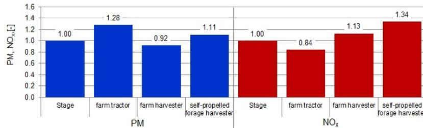
Figure 14. Comparison of the relative exhaust emission of PM and NO<sub>x</sub> (under actual operation) with the emission limits.
