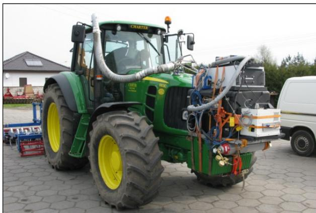
Figure 6. The view of the farm tractor with the measurement equipment.
