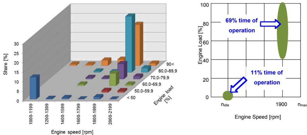
Figure 10. Time density characteristics and the most frequently used engine operating ranges of the self-propelled forage harvester.
