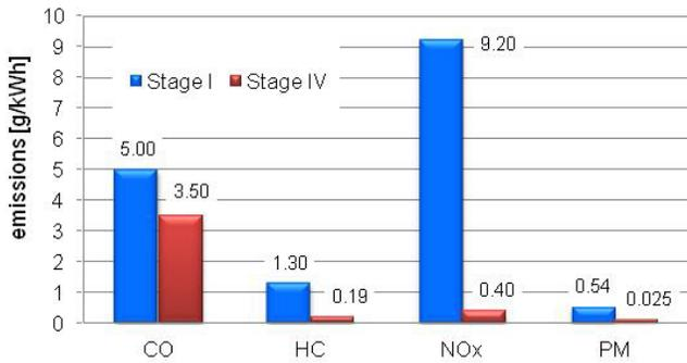
Figure 1. Comparison of the Stage I and Stage IV emission limits for non-road vehicle engines of the rated power of 130 to 560 kW.
