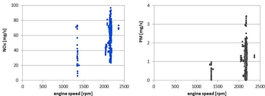
Figure 12. The emission of PM and NO<sub>x</sub> from the harvester.
