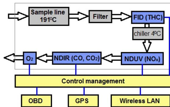
Figure 7. A diagram of a portable analyzer SEMTECH DS; exhaust gas flow channels (arrow) and electrical connections circled (blue line).
