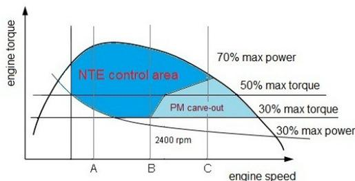
Figure 5. NTE control zone for U.S. engines, for C less than 2400 rpm (left) and for C greater than 2400 rpm (A, B, C - speed for the ESC cycle).
