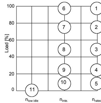
Figure 2. Diagram of the 11-phase test ISO 8178 (AVL, 2006).
