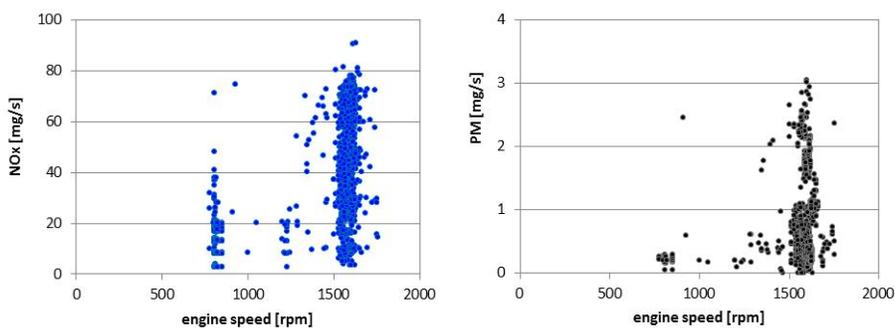
Figure 11. The emission of PM and NO<sub>x</sub> from the farm tractor.
