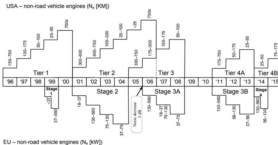
Figure 4. Exhaust emission standard implementation stages for non-road vehicles in the United States and Europe (AVL, 2006).
