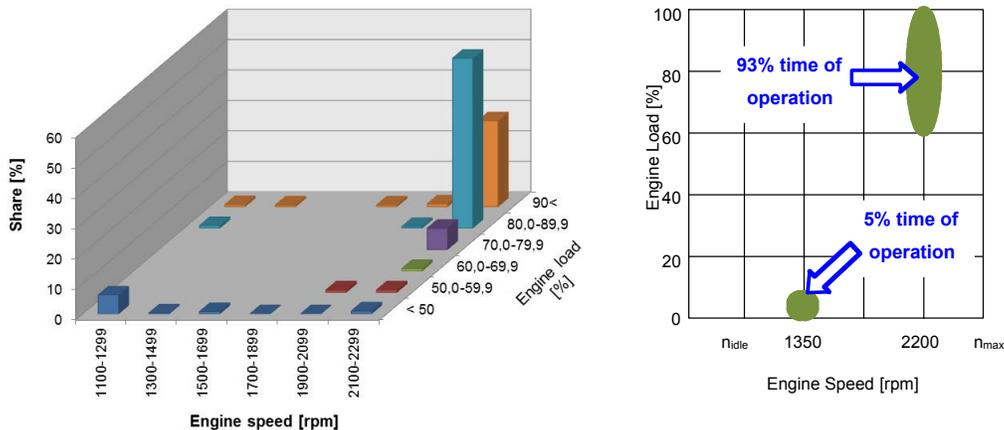
**Figure 9. Time density characteristics and the most frequently used engine operating ranges of the harvester.**
