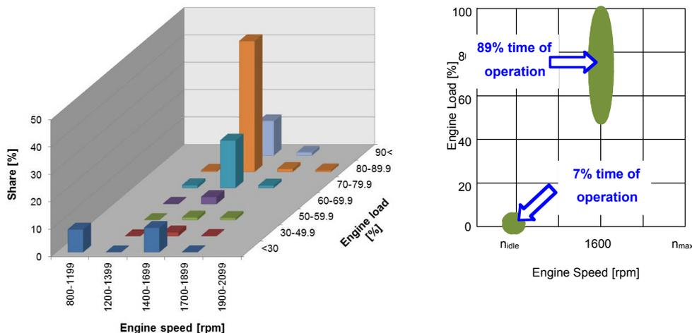
**Figure 8. Time density characteristics and the most frequently used engine operating ranges of the farm tractor.**
