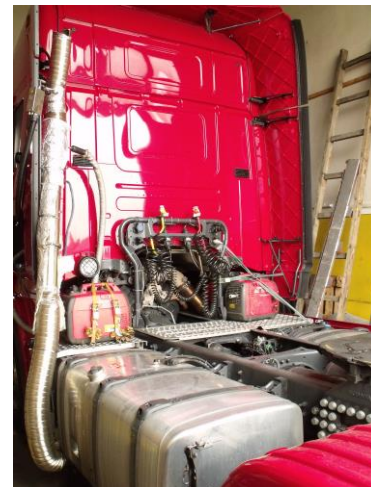
Fig. 4 The view of the exhaust sample uptake
